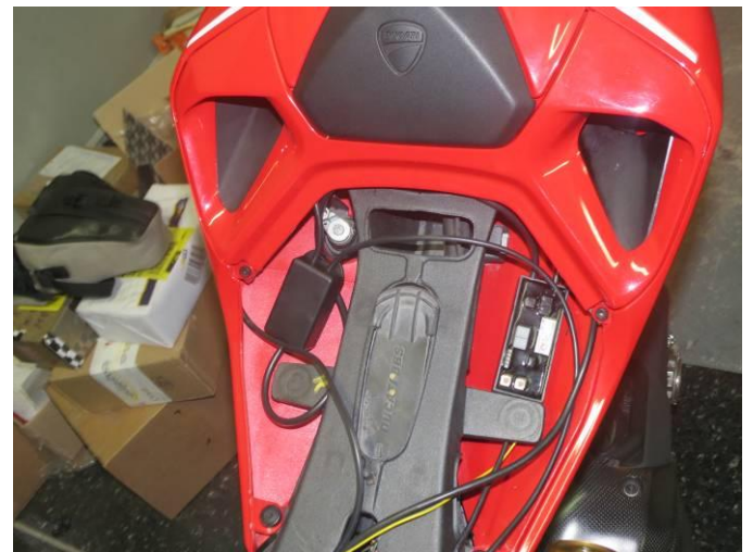
3.2 Load Cell installation
